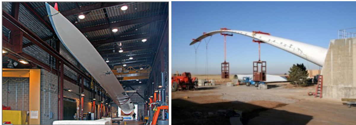
Photos 2 and 3 - Researchers conducting fatigue blade tests
